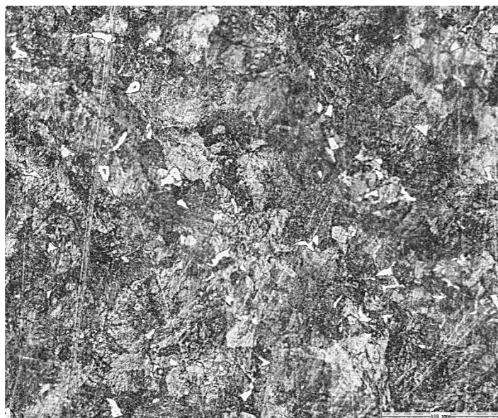
Figure 9 – Microstructure of the base metal of the templet (No. 1), x200
