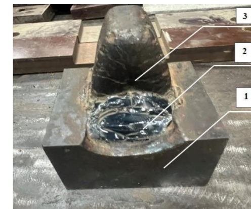
1 - the main metal of the gear, 2 – the area exposed to electro-slag surfacing (slag), 3 – the surfaced tooth
