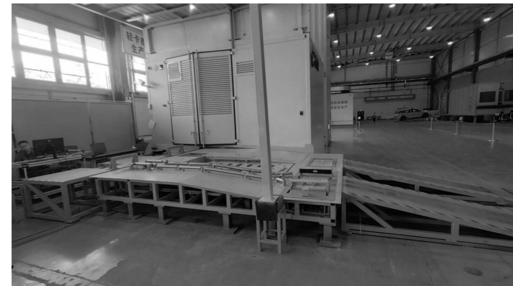
Figure 2 – Autonomous station for battery-swapping in small trucks
