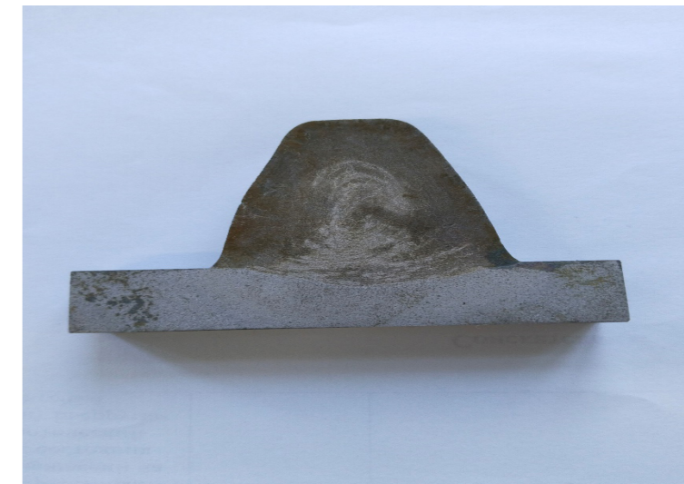
Figure 4 – Fragment of a deposited tooth with applied hardness values
