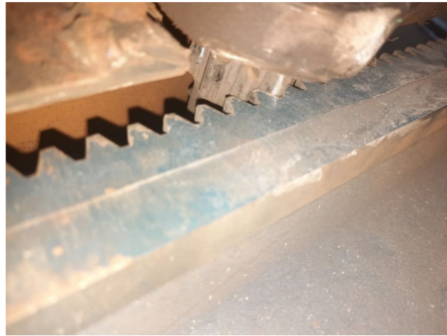
Figure 4 – Toothed rack of the plasma machine «KarPLAZ»
