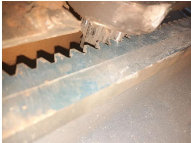
Figure 4 – Toothed rack of the plasma machine «KarPLAZ»
