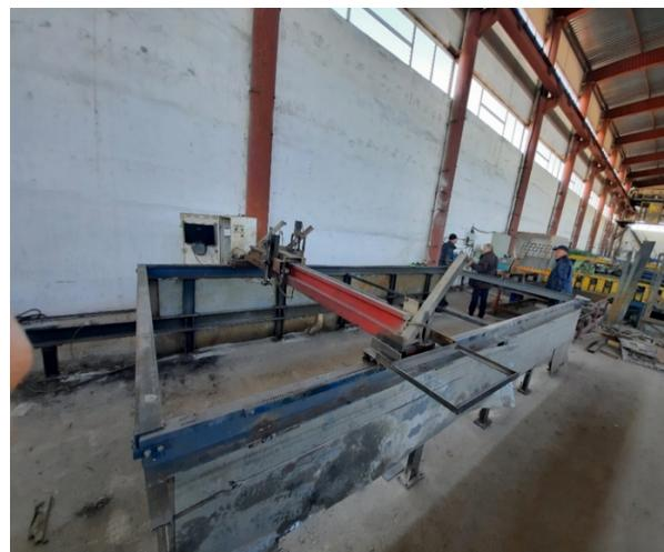
Figure 1 - Assembly of the plasma cutting machine «KarPLAZ»
