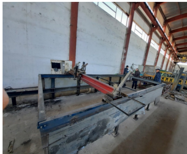
Figure 1 - Assembly of the plasma cutting machine «KarPLAZ»
