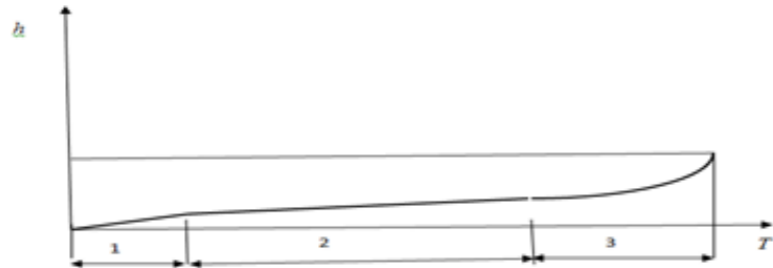
Figure 3 – Dependence of the rate of wear and corrosion on the aggressiveness of the medium
