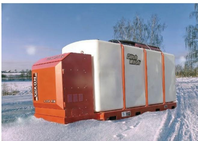
Figure 2 - “YUKON” drill mud heating unit
