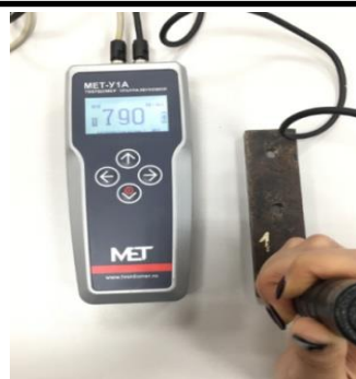
b) Vickers hardness measurement process
