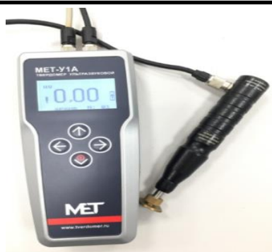
a) Portable ultrasonic hardness tester MET-U1A
