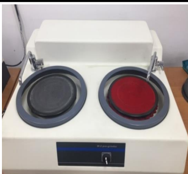
Figure 2 – Machine for preliminary grinding of metallographic specimens
