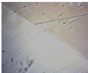
Figure 7 – Microstructure of diffusion layer of 65Mn steel samples after hardening
