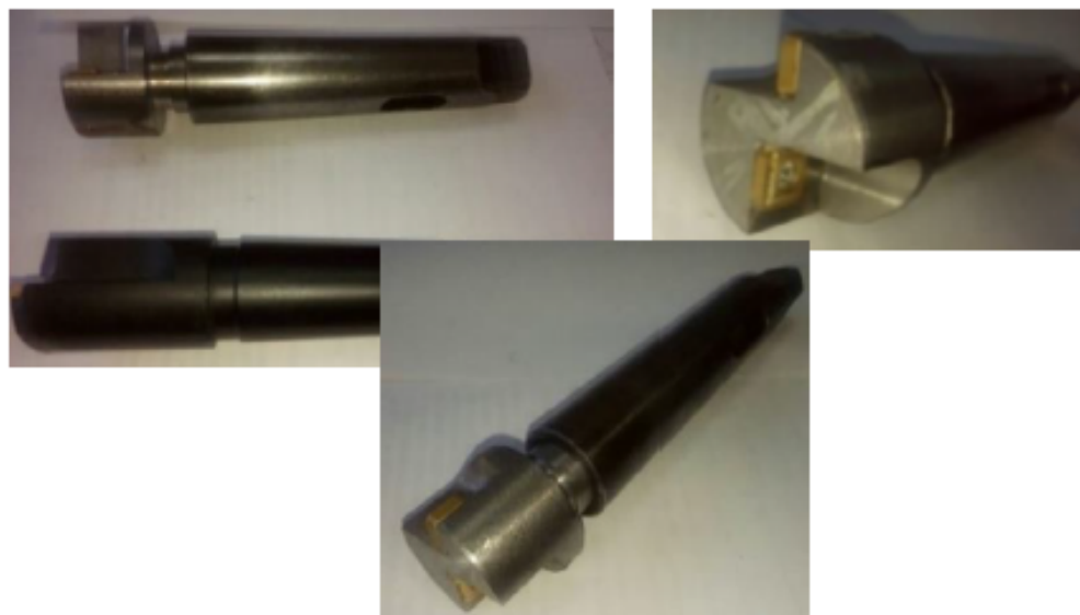
Figure 4 – Prototypes of combined cutting head
