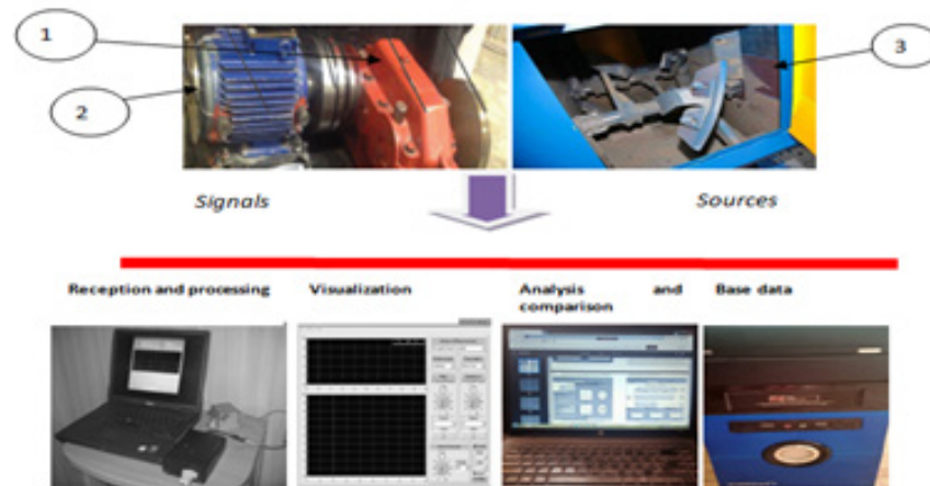
Figure 8 – Functional control diagram of the wear process of the mixer elements
