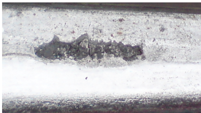
Figure 3 – Core fissures of VAE cross 60E1 1/11
