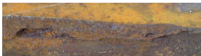
Figure 9 – VAE cross-cross R-65 1/11 detachment at Slampes station
