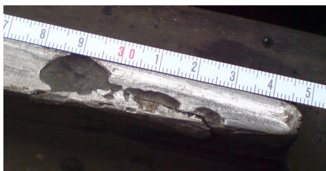
Figure 4 – Breaking of the core of the VAE cross 60E1 1/11 and cracks at the Alotene station
