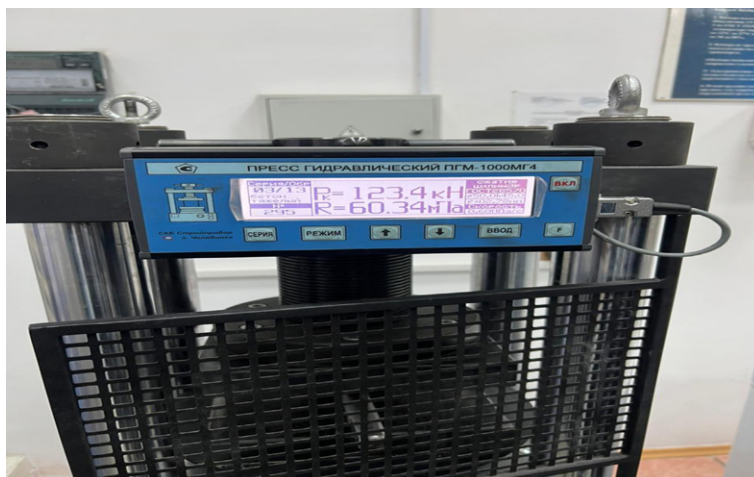
Figure 3 – Results of measuring the fracture force of cast iron casting
