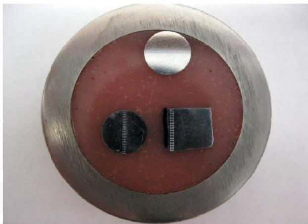
Figure 4 – Samples of aluminum alloy 7075 for microhardness test
