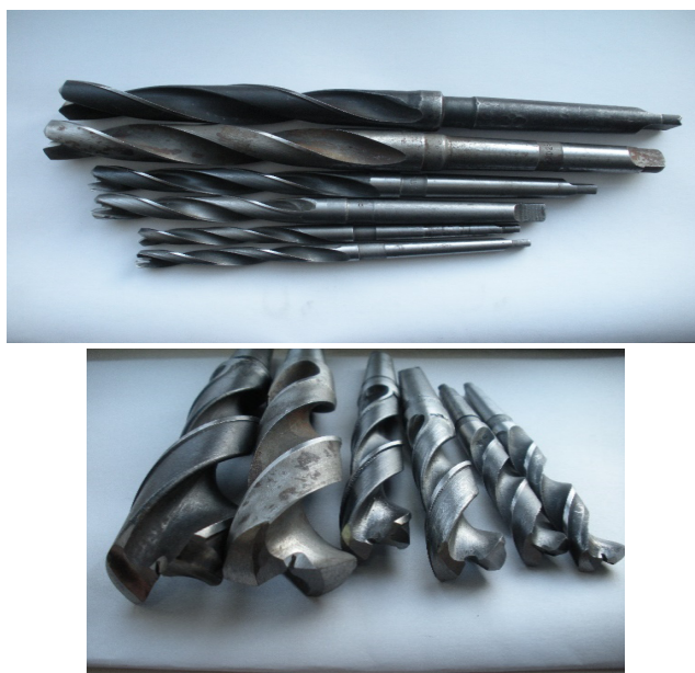
Figure 2 – Designs of double-ended spiral drills without a transverse edge
