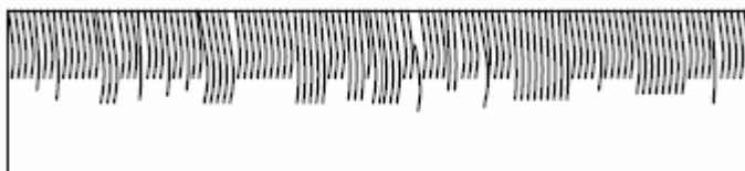
Figure 2 – Poor quality of the cut with noticeable notches and chips
