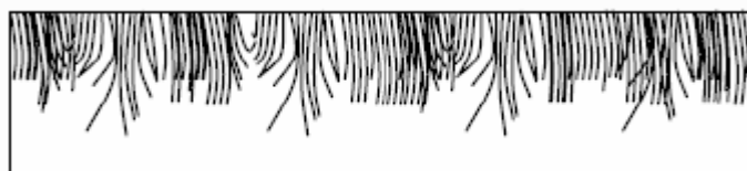
Figure 3 – Very bad cut with notches, chips and a jagged edge
